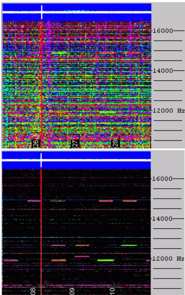
The pretrigger was set to 1 second for this test, so the trigger pulse is visible on the blue amplitude bar. The VLF [RDF antenna](#) was deliberately placed in a noisy environment (indoors), so the ALPHA pulses were barely audible in the noise. The waterfall 'contrast' was set to a high value; the same settings were used for both screenshots.
